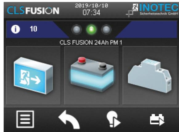
**!** If you are in the detailed view of a CLS FUSION system, you cannot start luminaire, device or module programming. These device-specific changes always have to be made directly on the particular CLS FUSION system.
