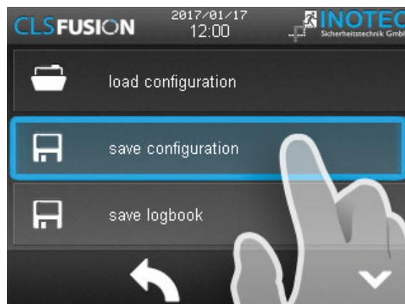
The configuration file gets saved on a USB port. The file name is Conf\_CLS(Date)(Time).cfg and can be altered and printed out with the INOTEC configuration software. As soon as the notification “The configuration gets saved” is closed, the USB port can be removed.
