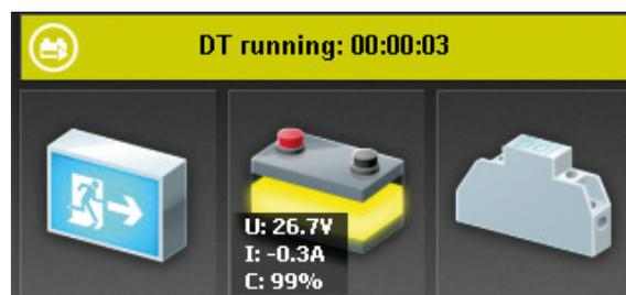
Once the DT has been concluded, the device switches back to normal operation mode. An active DT can be cancelled by activating the
