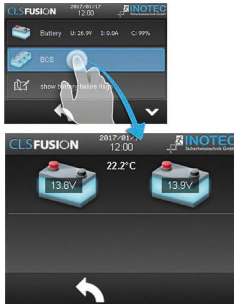
The sensors are displayed in separated columns with current values of the battery blocks which need to be monitored. Data about block voltage and temperature are listed here. To the left and right of the battery pair there are two coloured lines, which give the respective batteries their colour affiliations.
