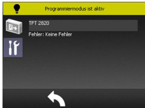
Luminaires with a grey background indicate luminaires that have not been registered or activated. Use the tool icon to log on to the individual luminaire classes. Click on the button with a light grey background (above "Failures: No failures") to go to the destination assignment.
