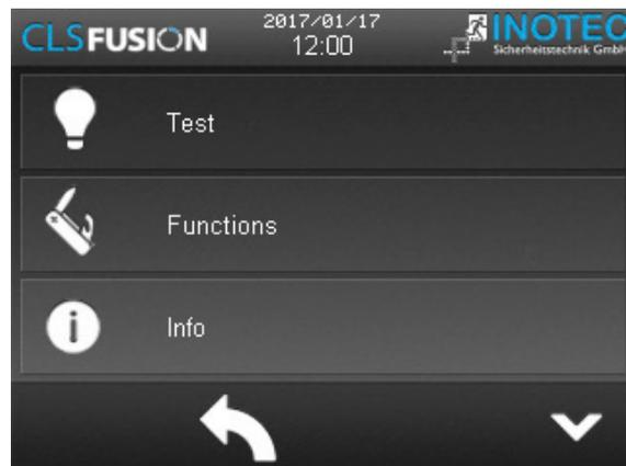
It contains various applications for systematically querying of the device status, testing possibilities and device settings. By activating the respective sub-menus, you can load/save configurations or check the logbook. When a setting is changed, it must always be saved or discarded. These two options appear automatically. To save the setting, click the floppy disk, and to discard it, click the dustbin.
