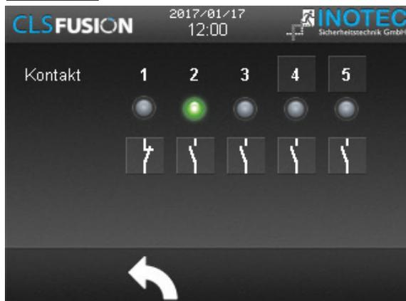
The system status gets displayed for the first three LED's. The relaisinterface is programmed at the factory. The notifications of the first three relais contacts are set up fixed (disruption, operation, battery operation). Check-boxes are below the luminaires. Here you can choose between make contact and break contact.
