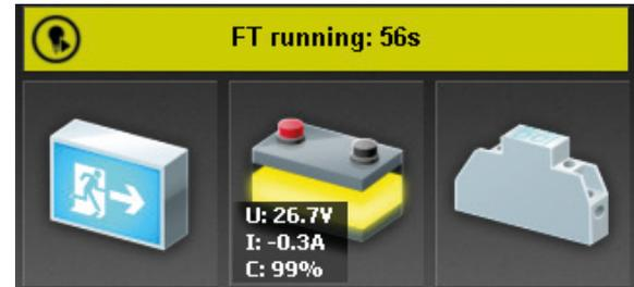
The device switched into the battery operation in the function test mode and tests the registered luminaires on functionality. The outcome of the function test gets saved in the logbook. The current status gets displayed in the “Status display” in the main menu. In case there is a current luminaire failure, this failure gets displayed. The status display as well as the luminaire symbol switch into the red colour mode.
