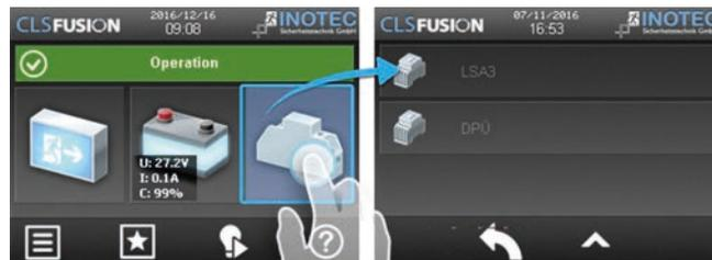
Submenus will show information about all connected DPÜ/B modules including their locations when you activate the button „Components“. All phases which were detected as a power failure will be highlighted by red LEDs in the submenu „DPÜ/B“.
